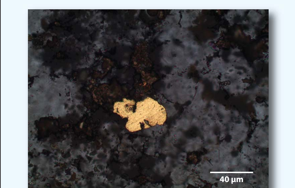
Combined reflected/plane light: Microscopic visible Au-Ag found in silicified organic-rich domain of vein breccia.
